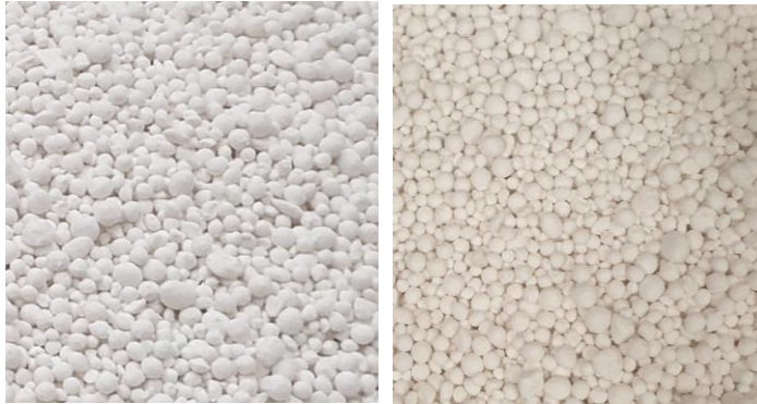
Granulated struvite taken from early tests
